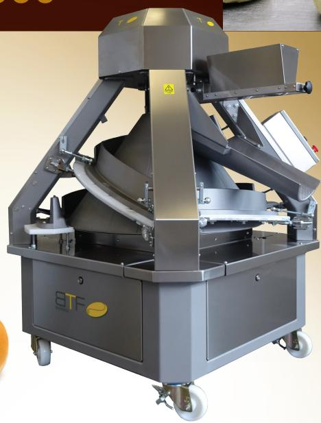
The conical rounder is ideal for rounding both soft and medium doughs. Rounding is achieved by a rotating cone, which rotates the dough along concave channels to produce roundly shaped dough.
